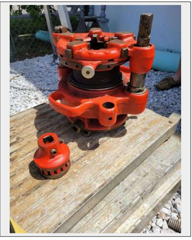
**Description** Rigid model 141 receding geared threader, for 2 1/2" - 4" pipes **Quantity:** 1
