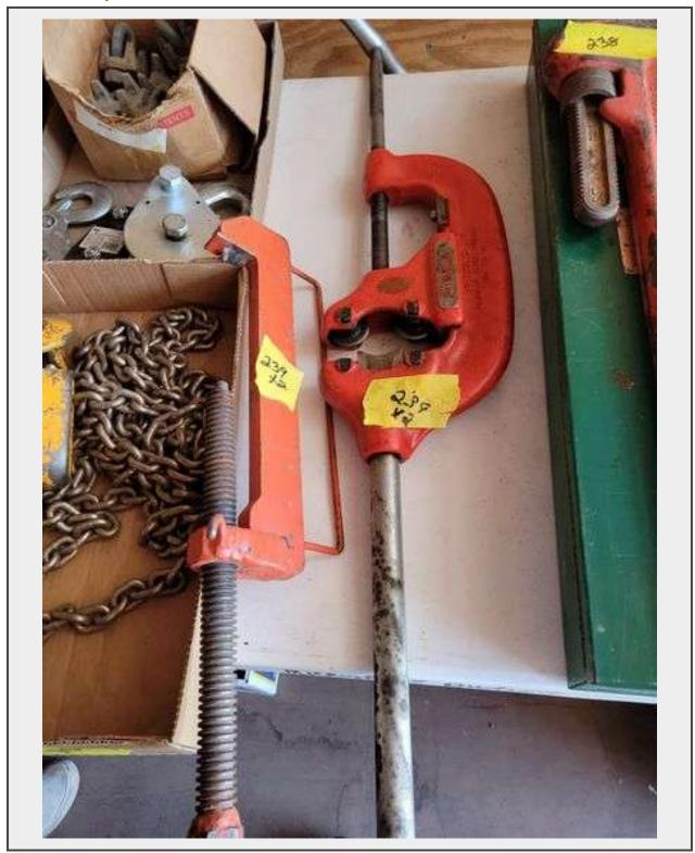
**Description**Rigid 2 1/2"-4" pipe cutter and pipe clamp
